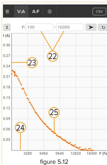
22. The range of frequencies for which the amplitude-frequency characteristics will be constructed.
